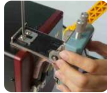
2. Tighten the screws. (Keep copper wires separate)
