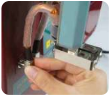
4. Insert the welding head into the corresponding socket.
