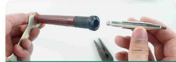
② Just insert the new electrode and twist it clockwise.
