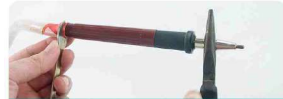
① Use a wrench to fix the nut at the end of the handle and use a sharp-nosed pliers to grip the electrode and twist it out counterclockwise.
