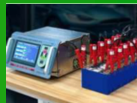
Equalizer repair Lithium battery pack
