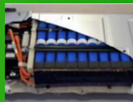
Lexus CT200h Hybrid battery module
